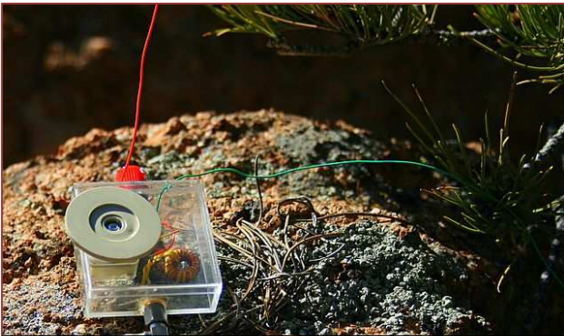
20m End Fed Halfwave tuner
