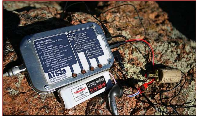
ATS3A with new label, lithpoly battery, ear bud and micro TENEKE paddle ready to rock!
