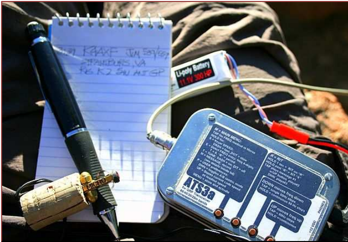
A 4-band ham radio station with manual logging software that fits on my lap.
