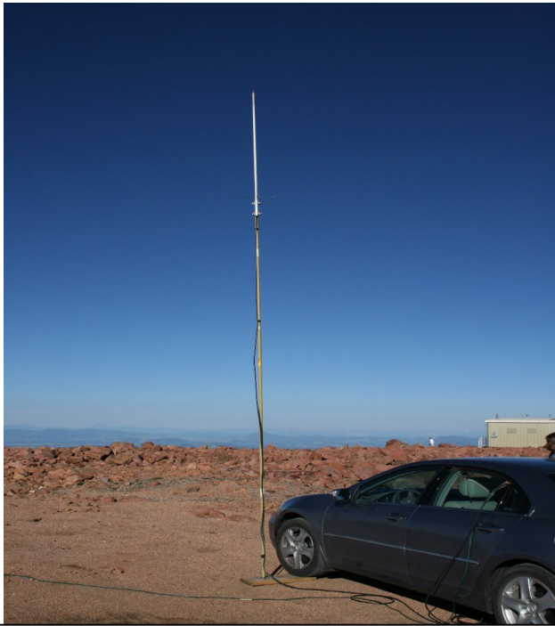
Drive on mount and mast with the X-50 antenna installed on top.
