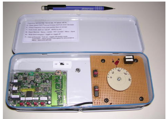
ATS-3 set-up – operating view
