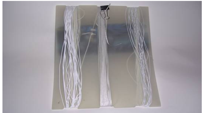
16-ft counterpoise, 45-ft end fed wire, pc board material clip board
